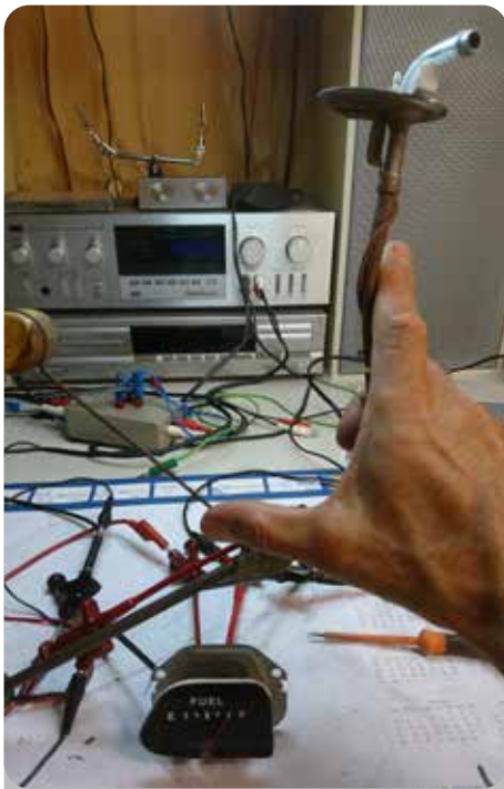
Sensor in positie tank vol
